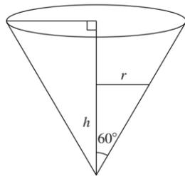
Step 1. The rate of change required is  $\frac{dh}{dt}$ , where  $h$  is the depth of the liquid.
